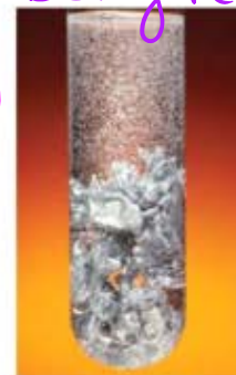
Figure 6.7B Zinc metal reacts with hydrochloric acid to produce zinc chloride and hydrogen. The bubbles shown here are hydrogen bubbles.
