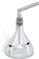
Charging an electroscope by conduction
