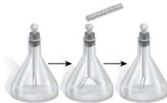
Charging an electroscope by induction
