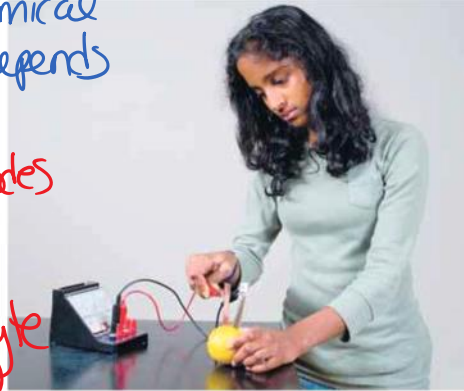
Step 3 Touch the leads from the voltmeter to the two strips.
