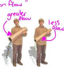
Figure 8.18 Even though both tubes have the same potential difference, the tube on the left has a greater "current" of marbles.
