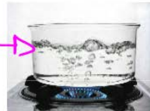
Figure 2.1.6 Vigorously boiling water. The bubbles are rising to the surface without collapsing.
