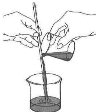
Figure 4B-3 When decanting, it is helpful to direct the liquid into the second beaker along a stirring rod, as shown here.
